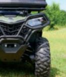
Fits MY 22-23 CFORCE 400 & 500 • Built with 1.25-inch/32mm-thick powder-coated steel Easy mounting with 4 strong mounting points
