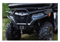
**FRONT BUMPER** Fits MY 20-23 CFORCE 600 & 600 Touring • Built with 1.5-inch-thick powder-coated steel Easily mounts to existing points/brackets
