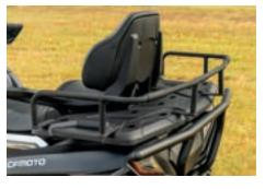
**REAR RACK EXTENDER** Fits MY 20-23 CFORCE 600 & 600 Touring • Built with 22mm-thick powder-coated steel Bolts easily into existing rack • Adds storage security on racks 9DS#-802400-6000 \$99.99 MSRP
