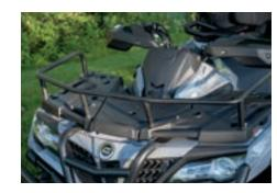
**FRONT RACK EXTENDER** Fits MY 19-23 CFORCE 800 XC, MY 22-23 CFORCE 1000 Overland • Built with 22mm-thick powder-coated steel • Bolts easily into existing rack • Adds storage security on racks 9AW#-802300-2000 \$99.99 MSRP
