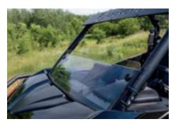
HALF FRONT WINDSHIELD, POLY Fits MY 23 ZFORCE 800/950 Trail, ZFORCE 950 Sport • Easy install with CFConnect system • Hard-coated, impact-resistant polycarbonate • UV protection to prevent yellowing
