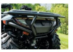
**REAR BUMPER** Fits MY 20-23 CFORCE 600 & 600 Touring • Built with 1.5-inch-thick powder-coated steel Easily mounts to existing points/brackets
