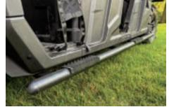
NERF BAR ASSEMBLY Fits MY 22-23 UFORCE 1000 XL Built with 2-inch-thick powder-coated steel
