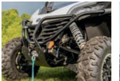
FRONT BUMPER Fits MY 21-22 ZFORCE 950 Sport, MY 22-23 ZFORCE 950 H.O. Sport/EX • Built with 1.5-inch-thick powder-coated steel Easily mounts to existing points/brackets
