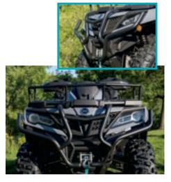
**FRONT BUMPER** Fits MY 19-23 CFORCE 800 XC, MY 22-23 CFORCE 1000 Overland - Built with 1.5-inch-thick powder-coated steel - Easily mounts to existing points/brackets - Provides full protection for front plastic and headliahts 9AW#-801100-2000 \$199.99 MSRP
