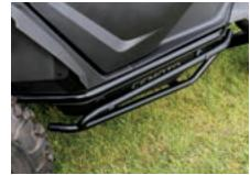
NERF BARS Fits MY 21-22 ZFORCE 950 Sport, MY 22-23 ZFORCE 950 H.O. Sport/EX • Built with 1.5-inch-thick powder-coated steel Easily mounts to existing points/brackets Provides protection for side plastics 5BY#-801300-1000 \$229.99 MSRP
