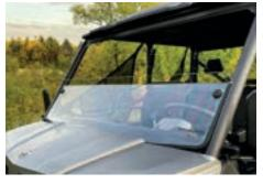
HALF FRONT WINDSHIELD, POLY Fits MY 19-23 UFORCE 1000, MY 22-23 UFORCE 1000 XL • Hard-coated polycarbonate screen • Quick, tool-less install with new clamp design Protects from outside elements 5SYV-805300-1000 \$239.99 MSRP
